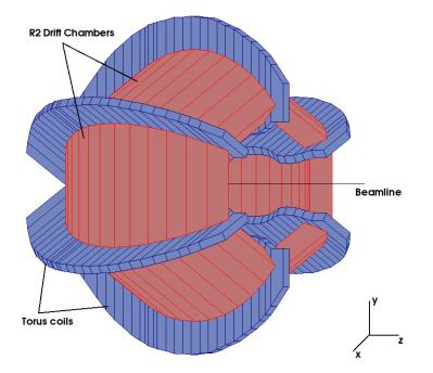
Figure 2.10: A drawing of the CLAS torus and R2 drift chambers, rendered in GEANT geometry.
