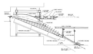
Figure 2.4: An engineering drawing of the photon tagger in Hall B. (Image source: [9]).
