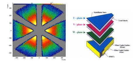
Figure 2.13: Left: A plot of electron occupancies in the EC looking downstream along the beamline. Warm colors indicate high occupancies. **Right:** A diagram of the u, v, and w geometry of a single sector of the EC. (Both images from [12])
