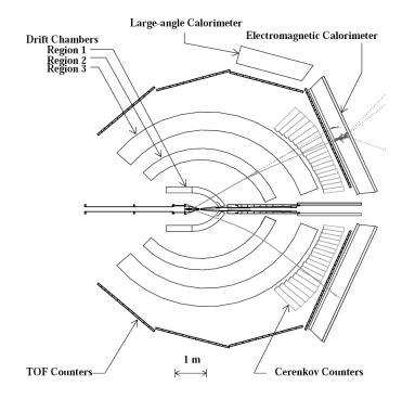
Figure 2.9: A diagram of the CLAS drift chambers.
