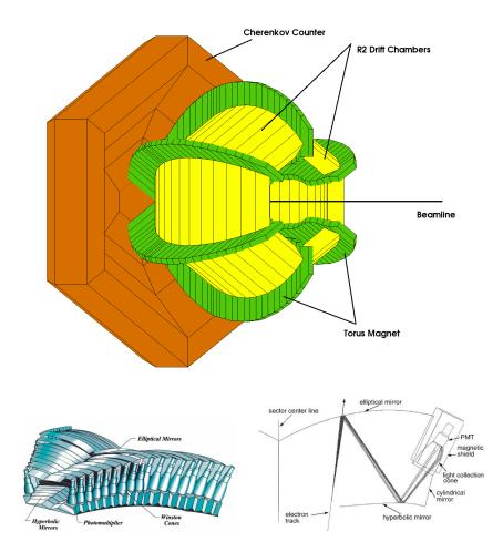
Figure 2.12: **Top:** A drawing of the CLAS Čerenkov counter, rendered in GEANT geometry with the R2 drift chambers and the CLAS torus to give a sense of scale and position. **Left:** Detail of the design of a single CC sector. Winston cones are devices that funnel light down into the phototube for more efficient collection (Image source: [11]). **Right:** Detail of the internals of a single CC mirror pair. The electron moves up the page. (Image source: [11])
