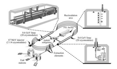
Figure 2.2: The components of CEBAF (Image source: [8]).
