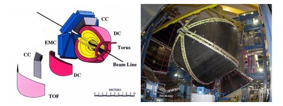
Figure 2.7: A cartoon showing the composition of the CLAS detector system (left); a photo of CLAS with the time-of-flight (TOF) withdrawn for service (right).
