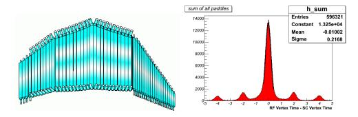
Figure 2.11: A drawing of a single sector of the CLAS time-of-flight (TOF) (left); the final g12 TOF timing resolution for pions (right). The secondary peaks at multiples of 2 ns are due to photons from different electron beam bunches.
